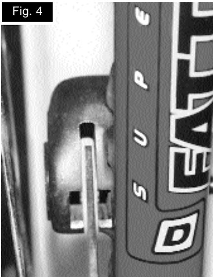
2. If the pads have been previously bedded in to the rotors and are simply being readjusted after brake bleeding or service, you should still screw in the fixed side pad adjuster just until it begins to slightly brush the rotor and then back it out counter-clockwise by quarter turns until the brushing sound stops. The fixed side pad must be set very close to the rotor for optimal brake power. Then set the piston side pad for desired brake lever travel and feel.
